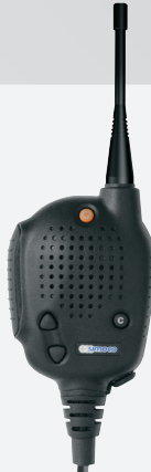
Remote Speaker Microphone RF antenna connector
